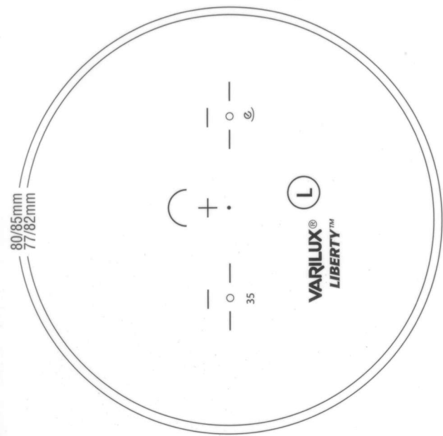
FIG. A. Fitting heights positioned too low can result in loss of useable reading area—one of the most common causes of non-adapts. To ensure proper positioning, place fitting cross marks over the midpupil. Check to be sure that the vertical fitting height is a minimum of 18 mm.
